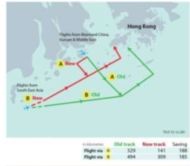
Illustrative diagram of new arrival tracks from north & west of Hong Kong
